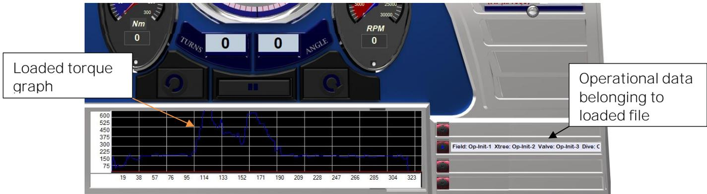
The loaded graph will appear in the graph window and torque-position ranges will be adjusted accordingly. Operational data for the loaded graph appears in the side window.
