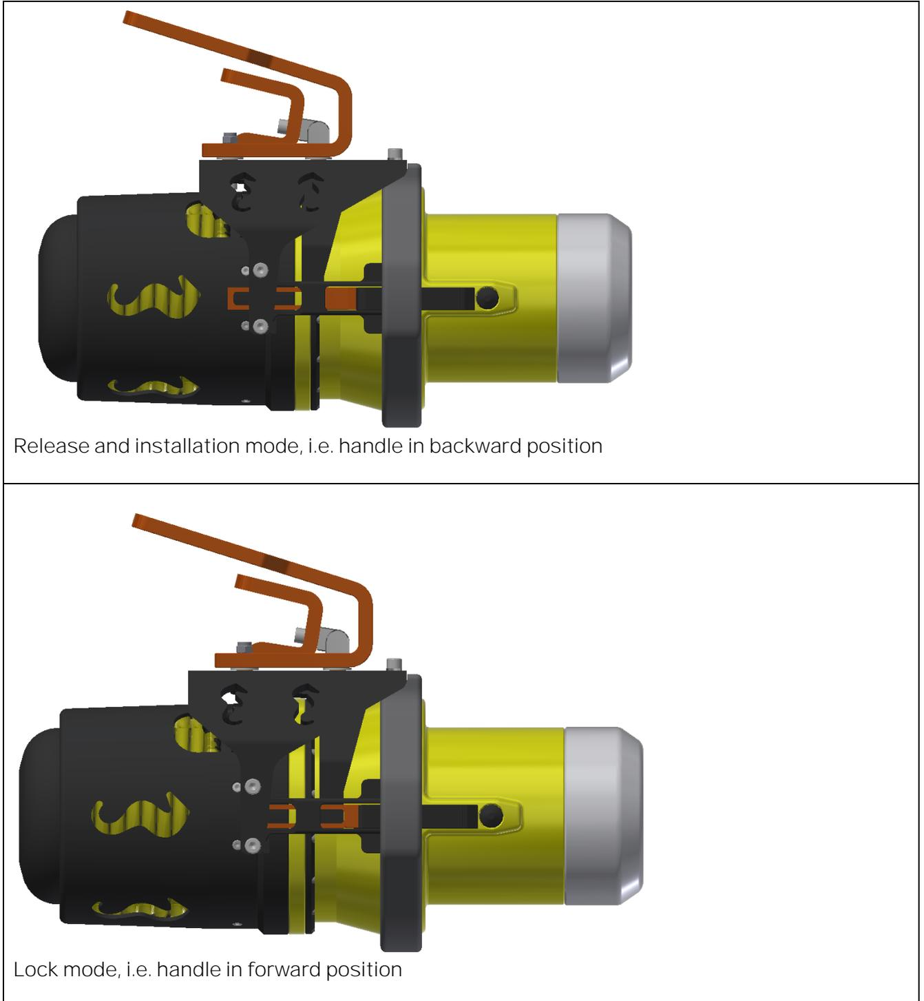
Figure 9, Locked and released mode
