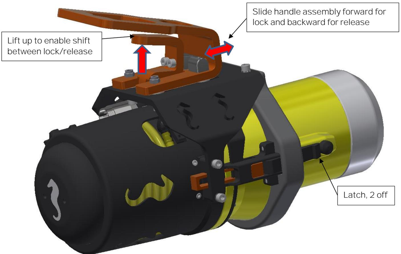
Figure 8, Latch mechanism
