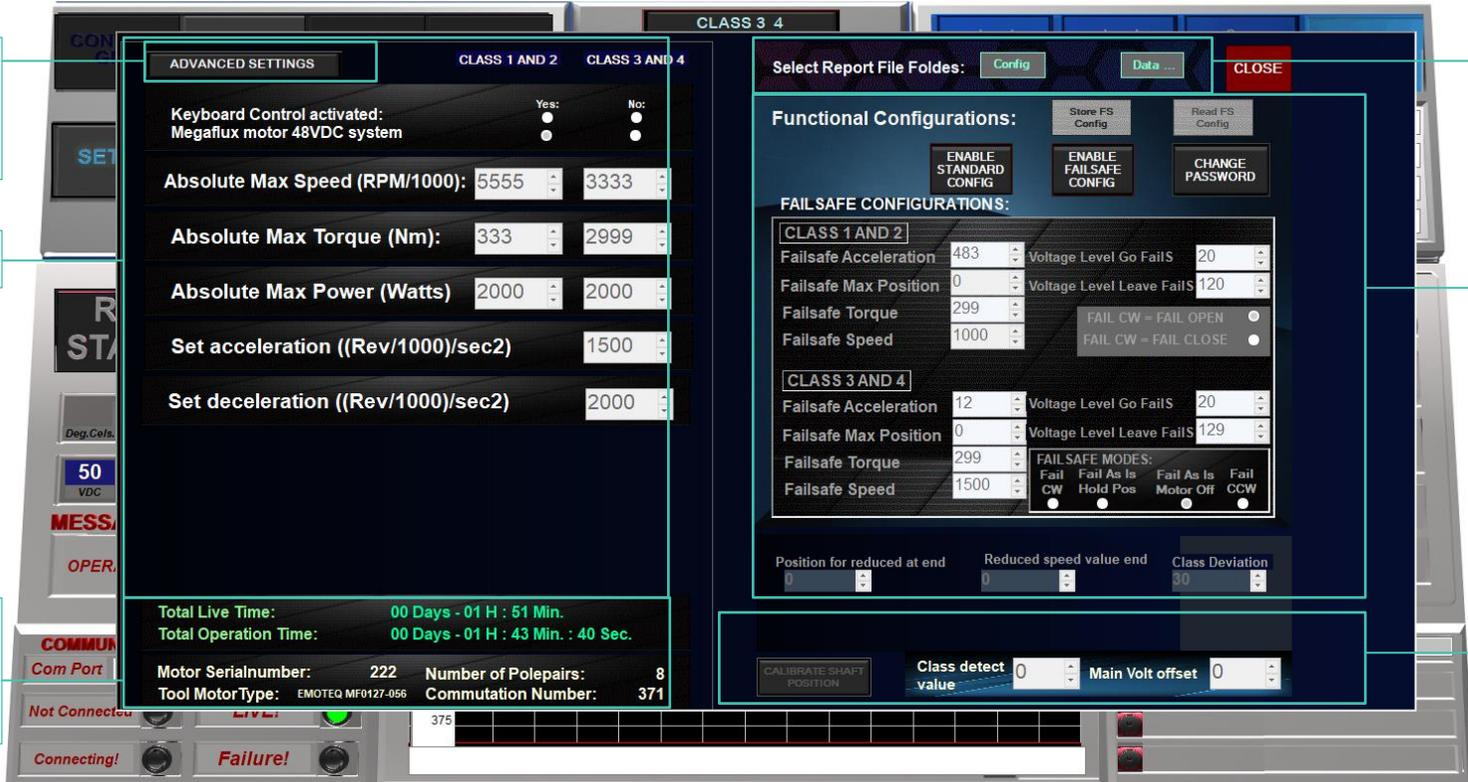
The screenshot shows the 'ADVANCED SETTINGS' window for 'CLASS 1 AND 2' and 'CLASS 3 AND 4'. The left panel contains performance and motor data, while the right panel contains functional and failsafe configurations. Callouts on the left point to 'Advanced settings (typical factory settings only)', 'Performance config', and 'Operation times and motor data (read only)'. Callouts on the right point to 'Archiving setup', 'Functional and Failsafe configurations', and 'Class and sensor factors'.
