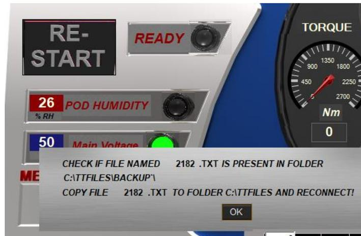
Overwrite the corrupt configuration file using the backup configuration file:
