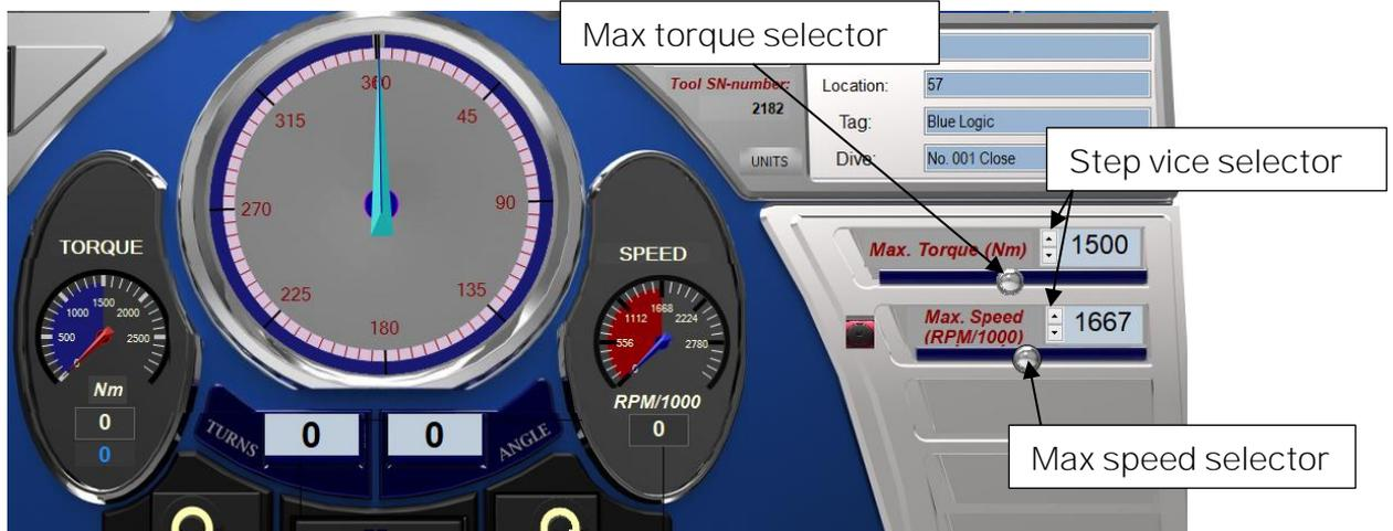
Adjustment can be performed by pressing and dragging the slider handles in the Operation Set Limit Board, or by clicking the one-step vice selector. Values can also be typed directly in the Operation Set Limit Board.
