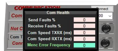
Receive Faults (%)      Number of data packets received but not approved by GUI
