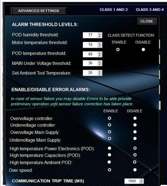
Advanced settings are factory settings for alarms. Alarm threshold levels These are levels that when reached will cause errors that shuts down operation to protect the system. Class detect function Here you can lock class and disable the class Detect function. If disabled class sensing will not occur but chosen class in “select class” will automatically be set.
