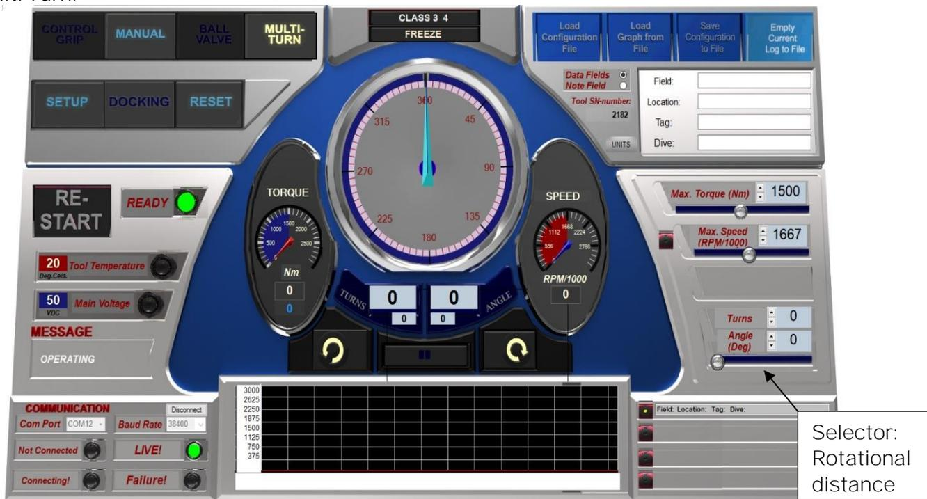
In Multi Turn mode the operator can select relative number of turns and rotational degrees the LWETT shall run before it stops. This mode is available first when reset are activated and all positions are set to zero. When in Multi Turn Mode a section in Operation Set Limit Board will appear where to set target position before operation. Set position is relative according to present position.
