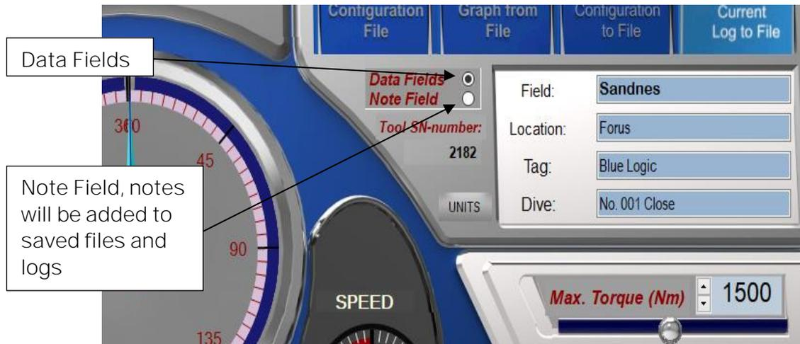
The following operations data may be typed in or imported by loading configuration file (See section 8.9.1).
