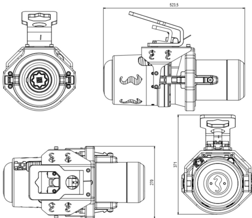
Figure 7 LWETT in ROV configuration - main dimensions
