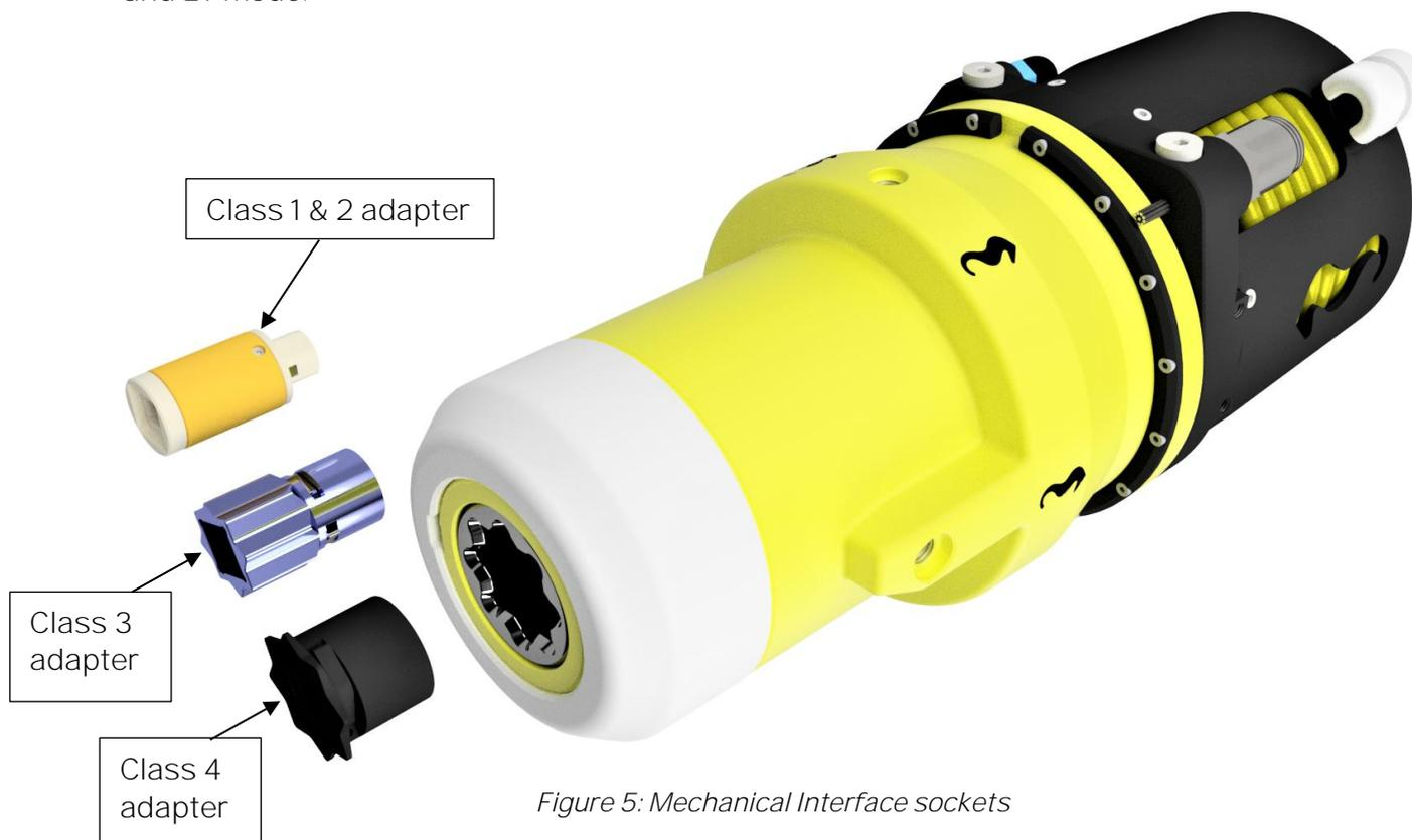
Figure 5: Mechanical Interface sockets
