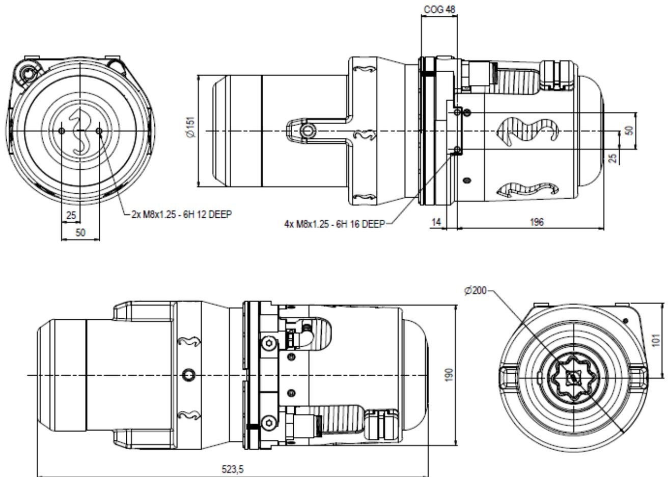
Figure 3, Torque Tool dimensions, AUV configuration
