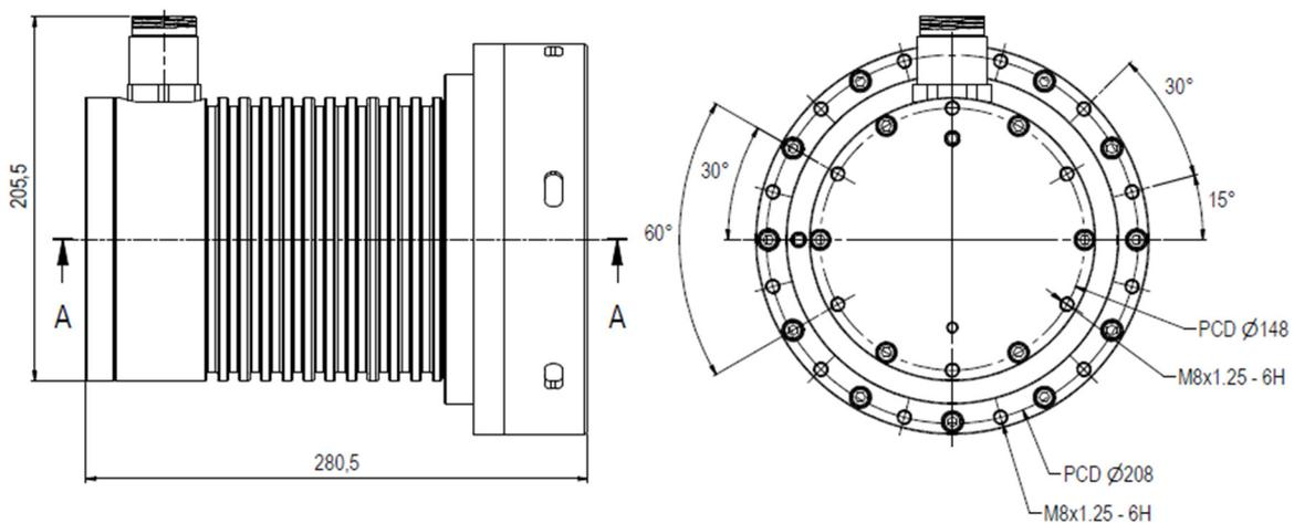
Figure 7 Secondary Connector Dimensions and Interfaces
