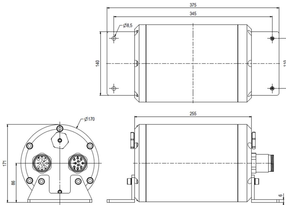
Figure 5 Power Factor Controller Installation interface
