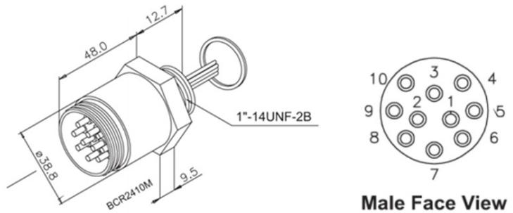
For prolonged used of the Primary Inductive Connector in seawater, adequate cathodic protection should be considered by the end user.
